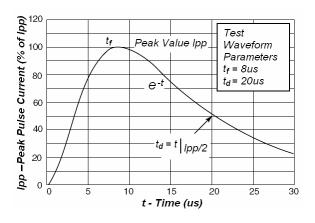
Fig1. Pulse Waveform
