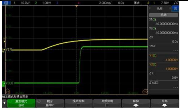
Vin=10V, Iout=30mA, Cout=10uF
