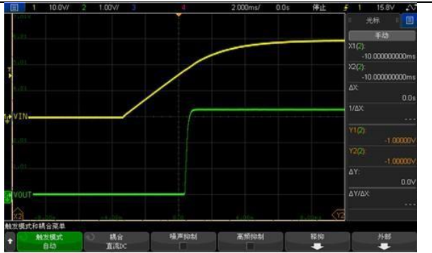
Vin=30V, Iout=0mA, Cout=10uF
