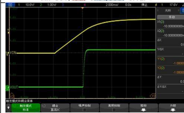
Vin=30V, Iout=30mA, Cout=0.1uF
